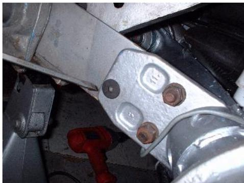
Second, the forward most spring plate-to-IRS arm bolt will have to be replaced with a flat head cap screw that must be countersunk into the flange on the IRS arm. This will prevent the tire from rubbing on the head of the bolt.
