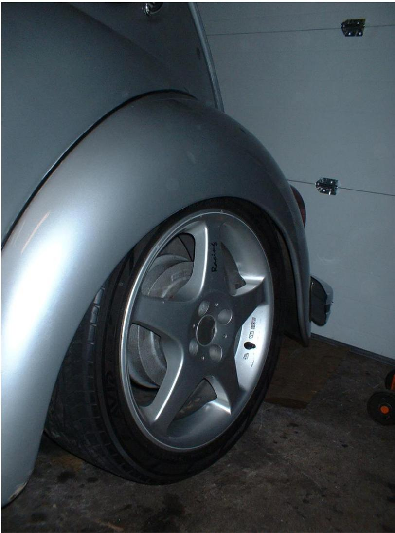
[caption: 16 x 7 +40 with 205/45 tires on on IRS rear suspension. Drum redrilled to 4-100mm pattern. No Spacers required.]
