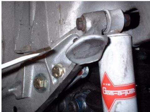
For the rear wheels, the rim will interfere in two locations and clearancing is required. First, the outermost  $\frac{1}{2}$ " –  $\frac{3}{4}$ " of the bumpstop plate has to be cut off.
