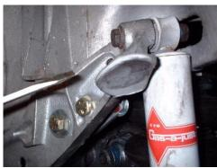
For the rear wheels, the rim will interfere in two locations and clearancing is required. First, the outermost  $\frac{1}{2}$ " –  $\frac{3}{4}$ " of the bumpstop plate has to be cut off.
