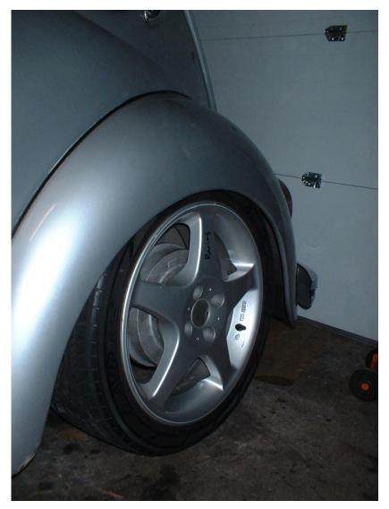
[caption: 16 x 7 +40 with 205/45 tires on on IRS rear suspension. Drum redrilled to 4-100mm pattern. No Spacers required.]
