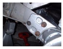
Second, the forward most spring plate-to-IRS arm bolt will have to be replaced with a flat head cap screw that must be countersunk into the flange on the IRS arm. This will prevent the tire from rubbing on the head of the bolt.
